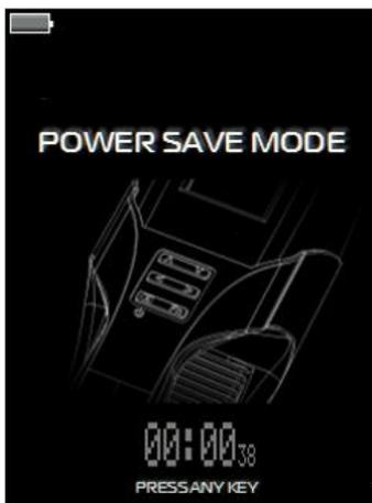
*Figure 14. Standby mode display of the device*
