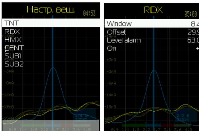
Figure 18. Setup Menu of substance identification parameters
