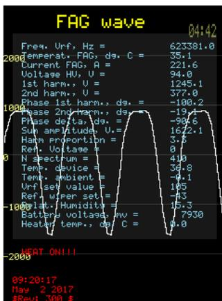
Figure 19. Oscillogram pattern of an asymmetric voltage generator with additional information on the operating mode of the device
