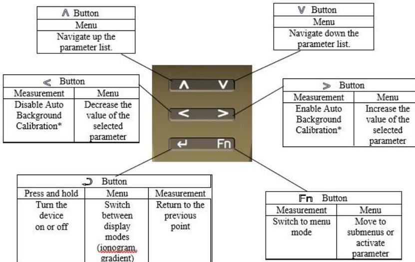
Figure 6. Description of the device buttons
