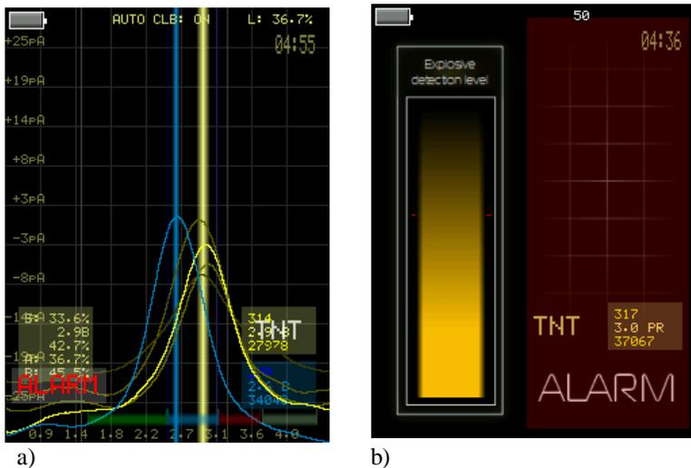
Figure 21. Weak signal for explosive vapors.
